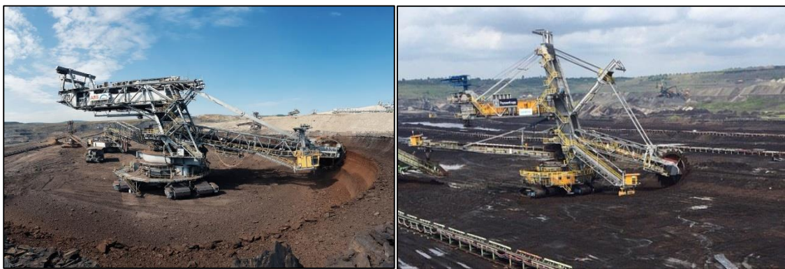
Figure 4. Rotary excavator on surface mining of coal in RB “Kolubara“, EPS, Republic of Serbia ( www.eps.rs. , 2024) and ( https://www.ekapija.com/ , 2023)
