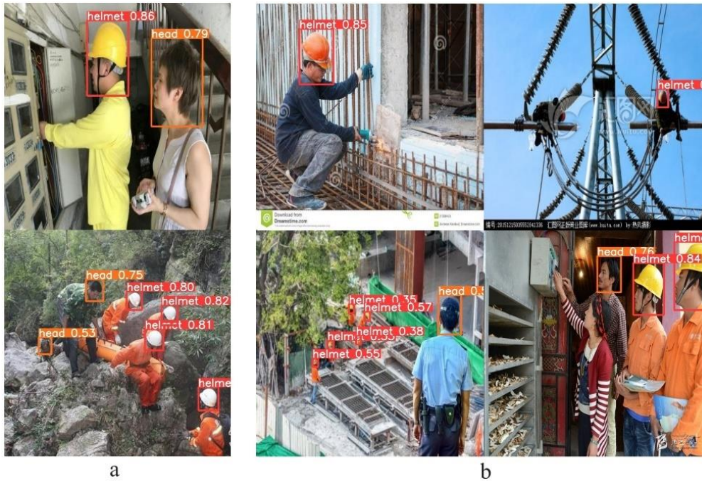
Figure 5. Examples of detection on the test set of YOLOv9e – a) examples of correct detection b) examples of incorrect detection
