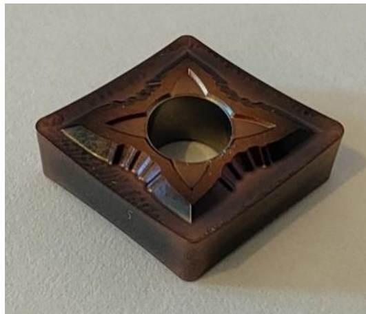
Figure 1. One of alternative cutting inserts: Pramet CNMG120408E-SF (nose radius r_e = 0.8 mm, rake angle of \gamma_{oi} = 14.5^\circ )
