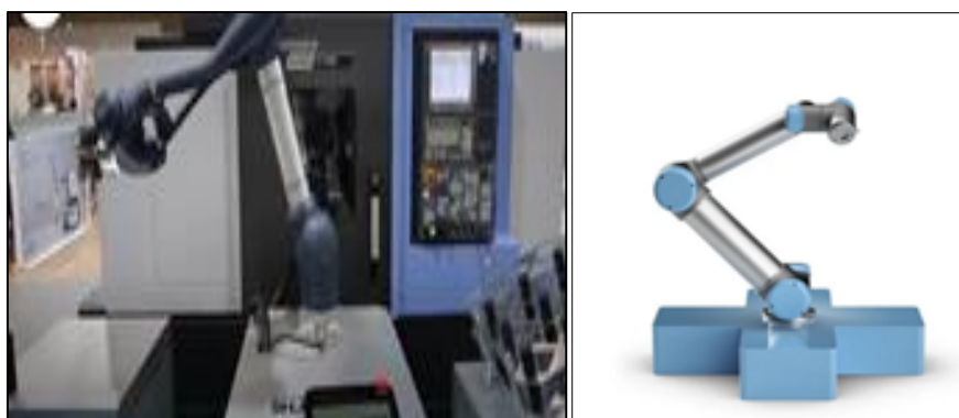
Figure 2. Display of collaborative robots intended for direct human-robot interaction within a common space, for Industry 5.0, ( https://qviro.com/product/universal-robots/ )
